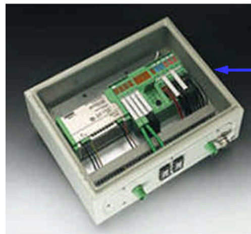
Distributed I/O Module Located Near Toll Lane
